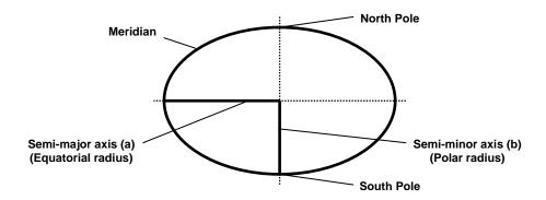
Geographical longitude and latitude are angular measurements. The longitude indicates an angle between the plane of the Prime meridian and the meridian passing through a point of interest. The latitude is the angle between the normal to the ellipsoid passing through the point of interest and the Equatorial plane (see figure below).
